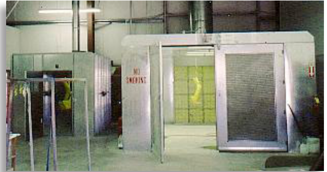
The area inside these spray and drying booths must be classified as Class I, Group B, C, or D locations.
