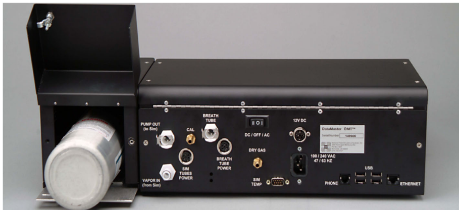
Image 2: Rear Panel of the DataMaster DMT with installed dry gas external standard tank.
