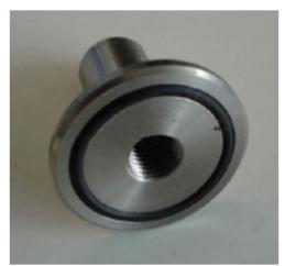
• After cleaning the rotor thread, apply a few drops of mineral oil (Anti-Corrosion Oil (rotor), cat. no. 9018543) on a soft, lint-free cloth, and wipe the thread. A thin, invisible oil film should cover the bucket mount and rotor claw, but no droplets or smear should be apparent.
