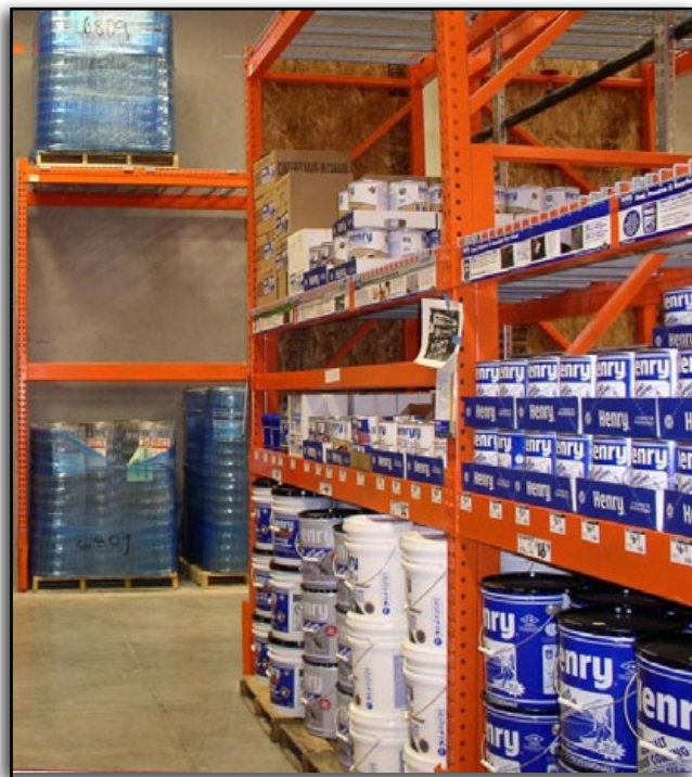
The hazard of these combustible liquids establishes the fire protection requirements.
