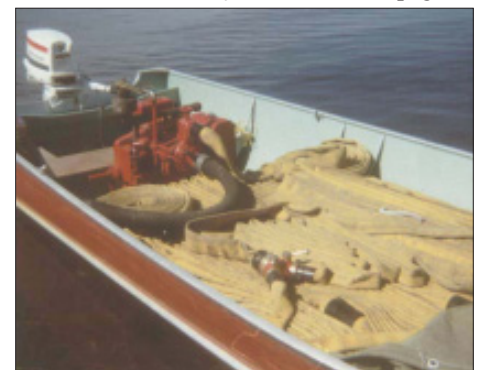
A village fire 'truck'. Where most travel is by waterway, a boat equipped with hose and pump is ideal.
