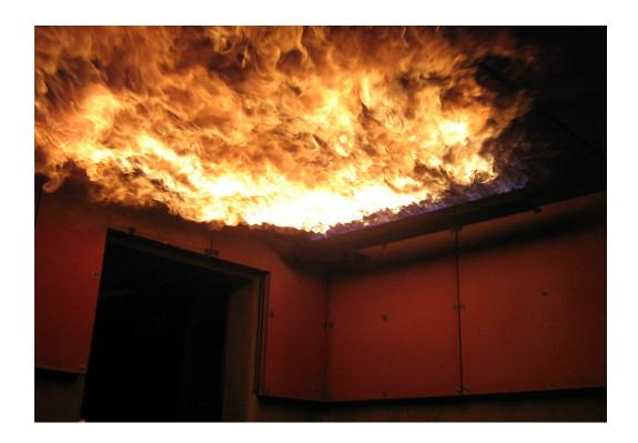
The **Second Story Training Room** includes a window with shutters, two (2) entry/exit doors to the front and rear open roof areas and an in-floor water bath burn pan, with living room furniture prop (chair). Students can be staged in front of, or behind the room for a starting point for evolutions, each path with a different approach to the stairwell. The room enables training in second story and basement training evolutions that start on the second floor and enter the burn chamber below.
