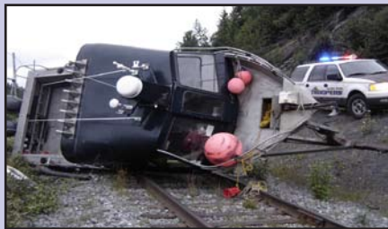
This 32-foot aluminum charter boat isn't trying to test its ability to navigate railroad tracks. Instead, it landed in the ditch of the Seward Highway after it came unhooked from the truck that was towing it in August. The incident was blamed on the improper ball size on the towing truck.
