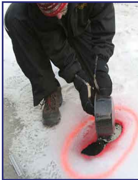
The technique involved pouring a molten sulfur compound onto a snow impression and developing an almost perfect replica of the impression.
