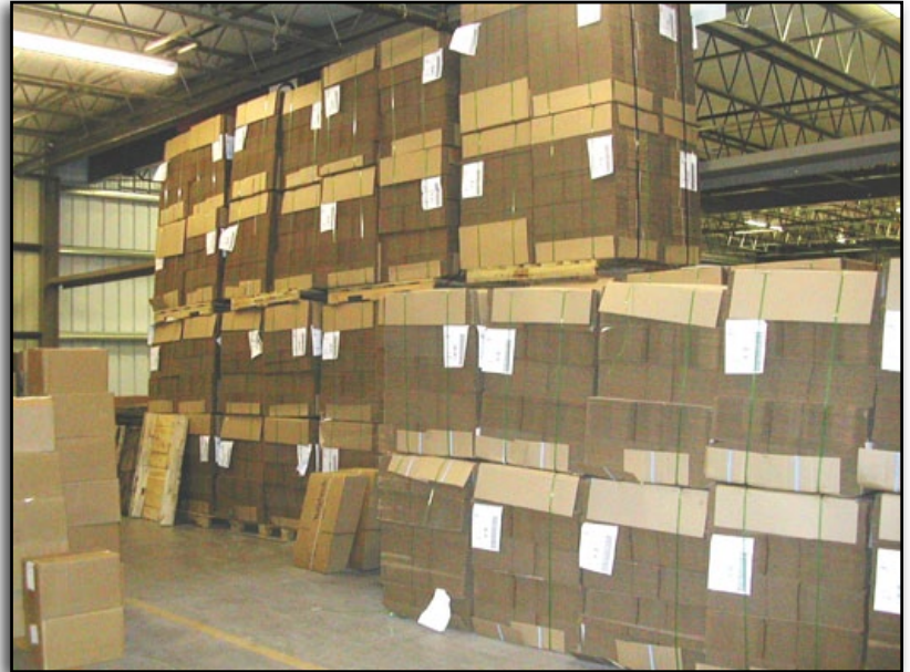
A “commodity” is the combination of the product being stored, its packaging, and the outer container in which it is located.
