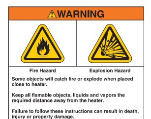
Clearances are the required minimum distances that combustible objects can be placed from the heater to prevent fire hazards. Combustibles are materials which may catch on fire and include common items such as wood, paper, rubber and fabric. Clearances to combustibles must be maintained at all times to ensure safety.
