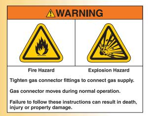
When connecting an infrared heater to the supply line, allowances for heater expansion are required. A flexible gas connector of approved type must be used. The gas piping system shall not bear any weight of any appliance. See NFPA 54/ANSI Z223.1 National Fuel Gas Code, latest revision.
